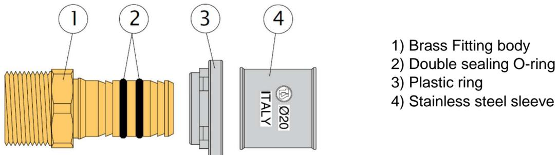
The body of the fittings (1) is totally made of brass with a complete range for most of the pipe sizes. The brass alloys that **te-sa** uses for the Press Fittings Series are suitable for uses in drinking water applications and compliant with the "4MS Common Composition List" and with the "UBA HCACL List".
